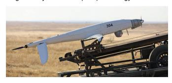
hybrid propulsion system featuring NWUAV's NW-44 Multi-Fuel Engine alongside an electric motor, the Skylark 3 Hybrid Small Tactical Unmanned Aerial System (STUAS) has tripled in endurance, without altering the size and weight of the aircraft. Offering up to 18 hours of operations, the Skylark 3 Hybrid offers RAF a more environmentally responsible UAV to help them achieve future capability ambitions.
