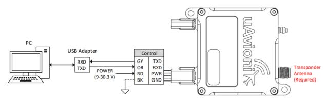
Set 'Conn Type' to 'Serial', 'Port' to the USB or serial port connected to ZPX-A, 'App Baud' to '57600' and 'Protocol' to 'UCP'.
