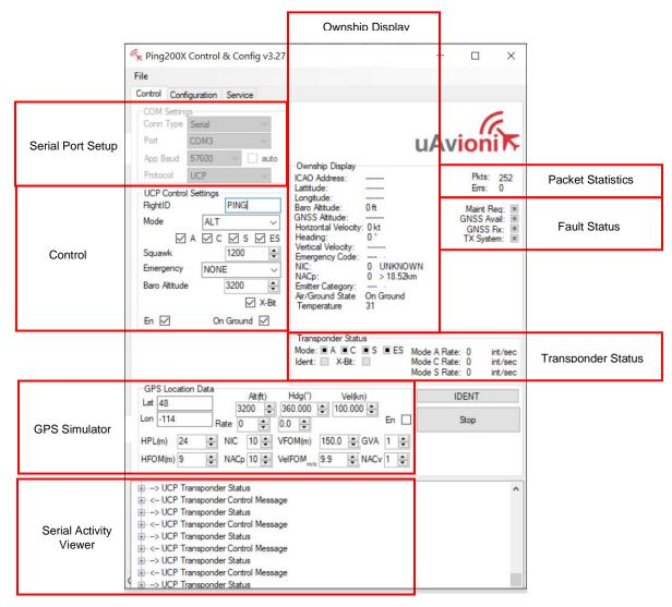
Note: Enabling X-bit produces a Mode A reply having X-bit = 1. In Mode S replies, X-bit = 0 (i.e., X-bit cannot be enabled for Mode S replies).
